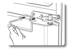
2. After removing one screw and two bolts, remove the Middle Hinge. (Unscrew the screws with the screwdriver(+) and hex bolts with the 4.75mm hex wrench.)
